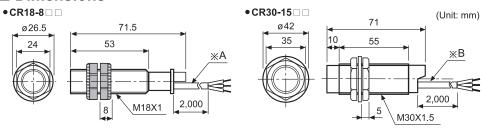
\*X'A' type: Ø4, 2 cores/Ø4, 3 cores(Conductor cross section: 0.3mm², Insulator diameter: Ø1.25)
